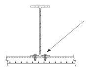
3/8" Bolt with washer and Nut (typical) by others. Drill 7/16" holes in steel and MOORFRAME.
