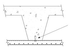
3/8" Hilti Kwik expansion anchor (B/O). Drill 7/16" Holes in concrete and MOORFRAME.
